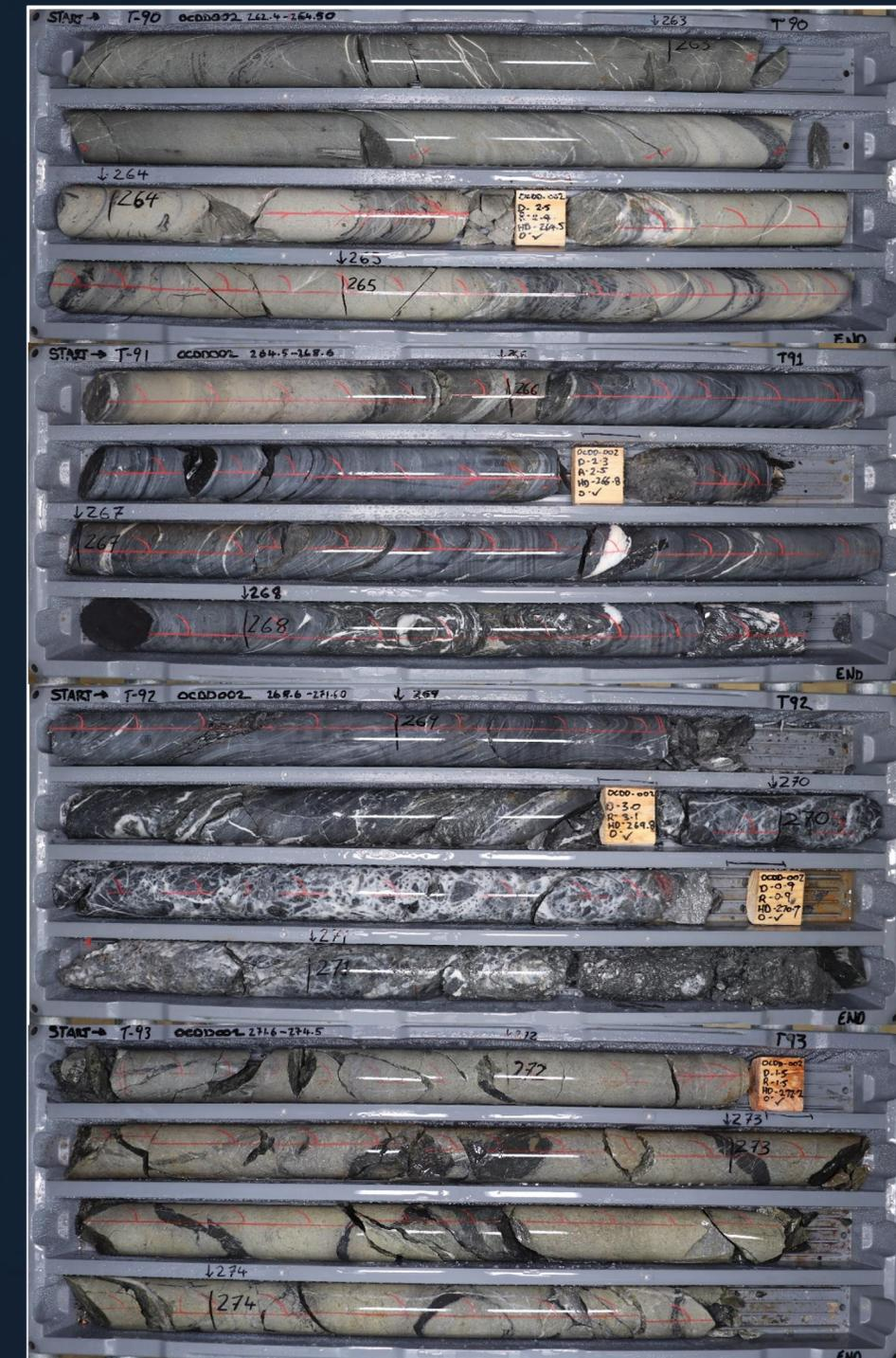
Figure 2 - Mineralised Parkes Shear OCDD002 (266.0-271.6m)
